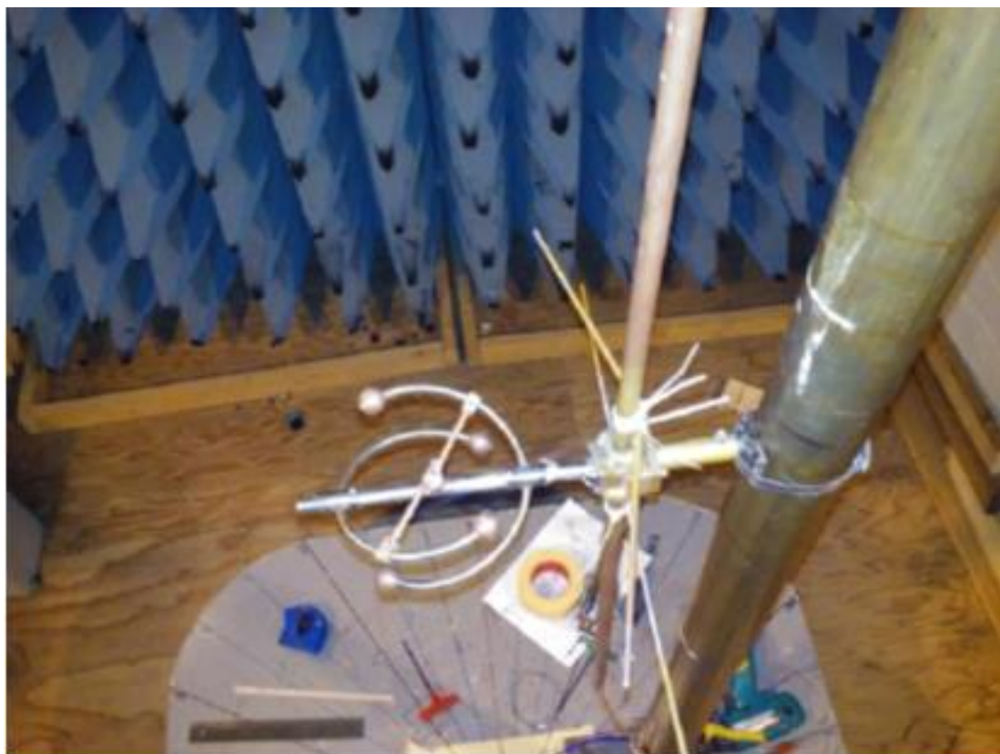
Figure 7 – Overhead View of Scaled Physical Model Used for Pattern Study in Anechoic Range
