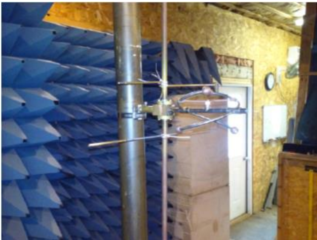
Figure 5 – Side View of Scaled Physical Model Used for Pattern Study in Anechoic Range
