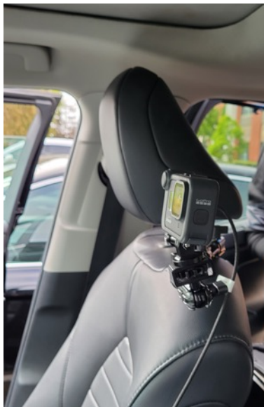
Figure 28. Photograph of GoPro Mount and Camera with Media Mod
