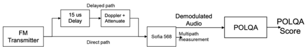
Figure 15. Lab Test System Block Diagram for POLQA Audio Quality Measurement
